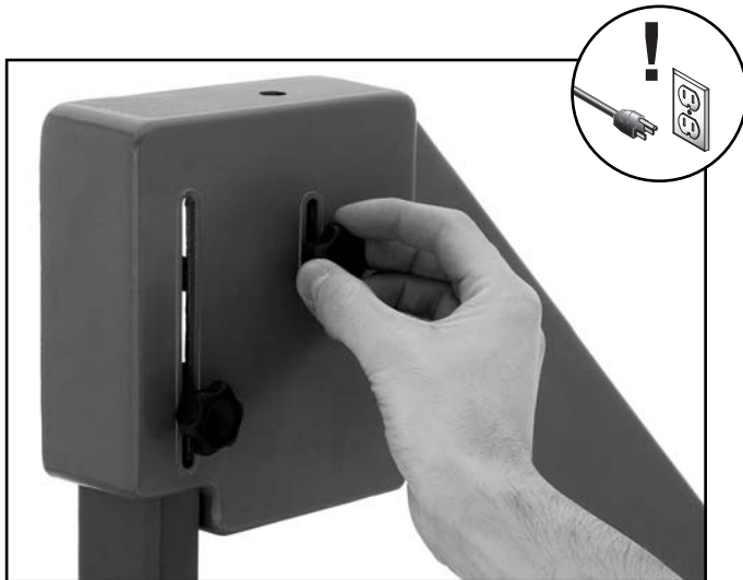
Figure 17. Loosening the wheel locking knob.
